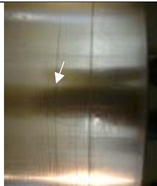
Fig.2: Close up view of crank pin journal showing deep scratch.
