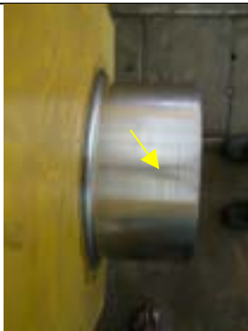
Fig. 1: crank pin journal portion showing scratch marks.
