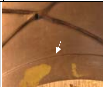
Fig. 5: Enlarged view of the bush bearing showing deep scratch mark at the bottom edge.
