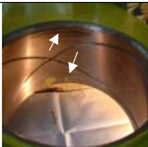
Fig. 4: Bush bearing with scratch mark at the lower end and dark adhesive wear patch at the top end.
