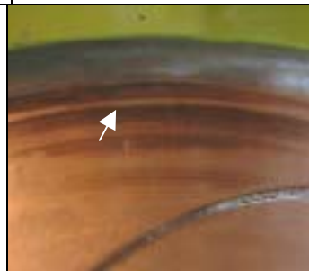
Fig. 6: Enlarged view of the bush bearing showing the black adhesive marks at the top edge.
