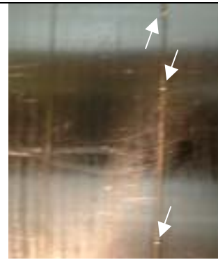
Fig. 3: Close up view of the scratch showing burrs adhering to the surface.
