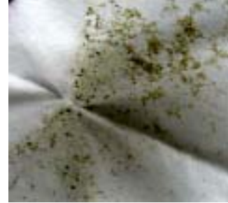
Fig. 9: Dust particles in the grease of LHS journal.
