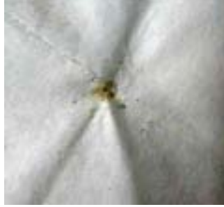
Fig. 8: Dust particles in the grease of the LHS bearing.
